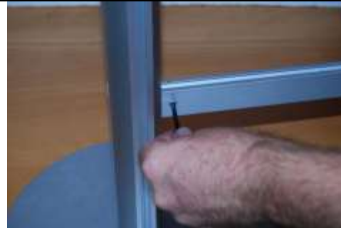
Step 4 Remove Top Pole caps and Insert Bottom Rail into Post slot. Once positioned, with clamp head located in slot, tighten the screw (clockwise rotation), repeat on the other post – adjust height to suit backing board
