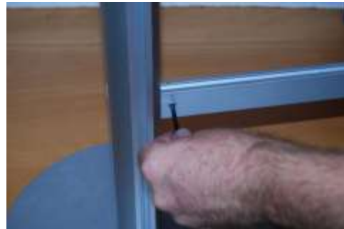
Step 3 Remove Top Pole caps and Insert Bottom Rail into Post slot. Once positioned, with clamp head located in slot, tighten the screw (clockwise rotation), repeat on the other post – adjust height to suit backing board
