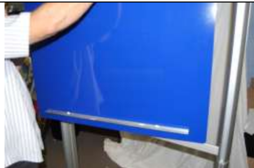
Step 5 Attach support rail to backing panel pieces and insert onto Bottom Rail
