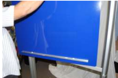
Step 4 Attach support rail to backing panel pieces and insert onto Bottom Rail
