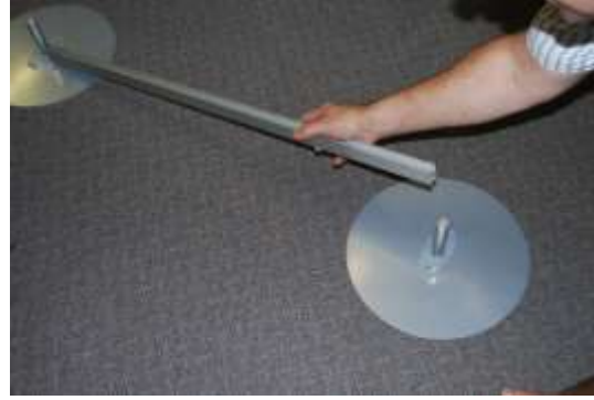
Step 1 Layout Bases and use one of the rails as a spacer to help locate position
